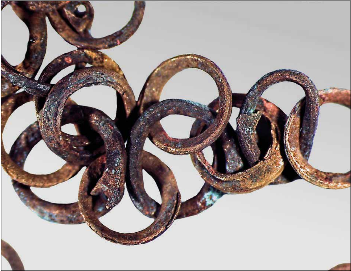
Fig. 8.14. Punching rings from sheet metal can result in conical-shaped solid rings, such as observed here in the solid rings of the hybrid armour from Newstead 4 in the United Kingdom. In addition to their conical shape, these rings also contain burrs from the punching action (photograph M.A. Wijnhoven).
