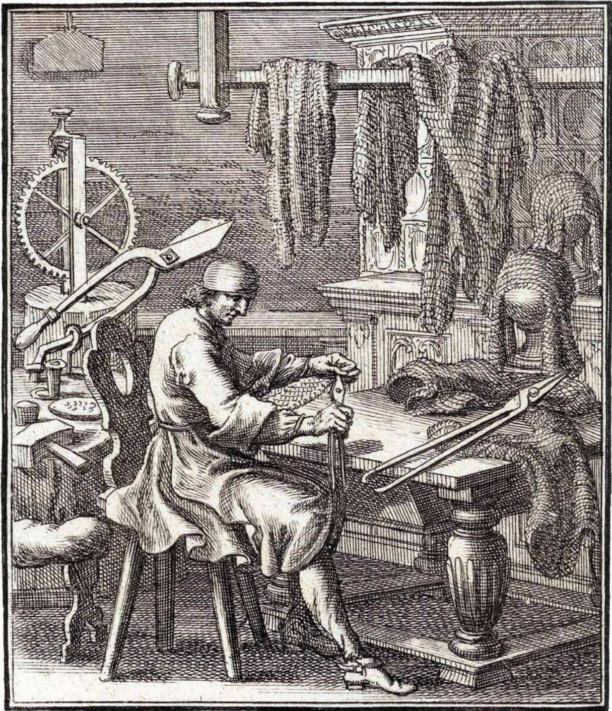
Fig. 8.4. The mail maker illustrated in Weigel's Book of trades . This copper engraving is the most detailed illustration of a mail maker's workshop. In the background there is a toothed wheel mounted on a stump, probably part of a mandrel (e.g. the gearing part) for coiling wire. A pair of large shears is mounted on another stump, next to one or two small anvils and a hammer. In the foreground the mail maker is shown seated behind his workbench weaving rings into a section of mail. A beam with several randomly arranged mail garments is located above the bench. Behind, there are two mounted wooden spheres, which could have been used for making mail coifs (Weigel 1698, M.A. Wijnhoven library).
