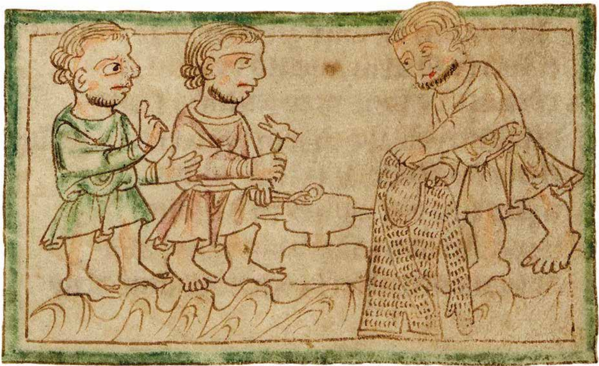
Fig. 8.2. The earliest image of a mail maker is an illumination from The romance of Alexander , dated around AD 1250. The mail maker works a ring on an anvil by holding it with a tong in one hand and wielding a hammer in the other. Facing him is a person holding the finished product, a mail hauberk that includes mittens and a hood. Cambridge University Library (MS O.9.34 – folio 24v).
