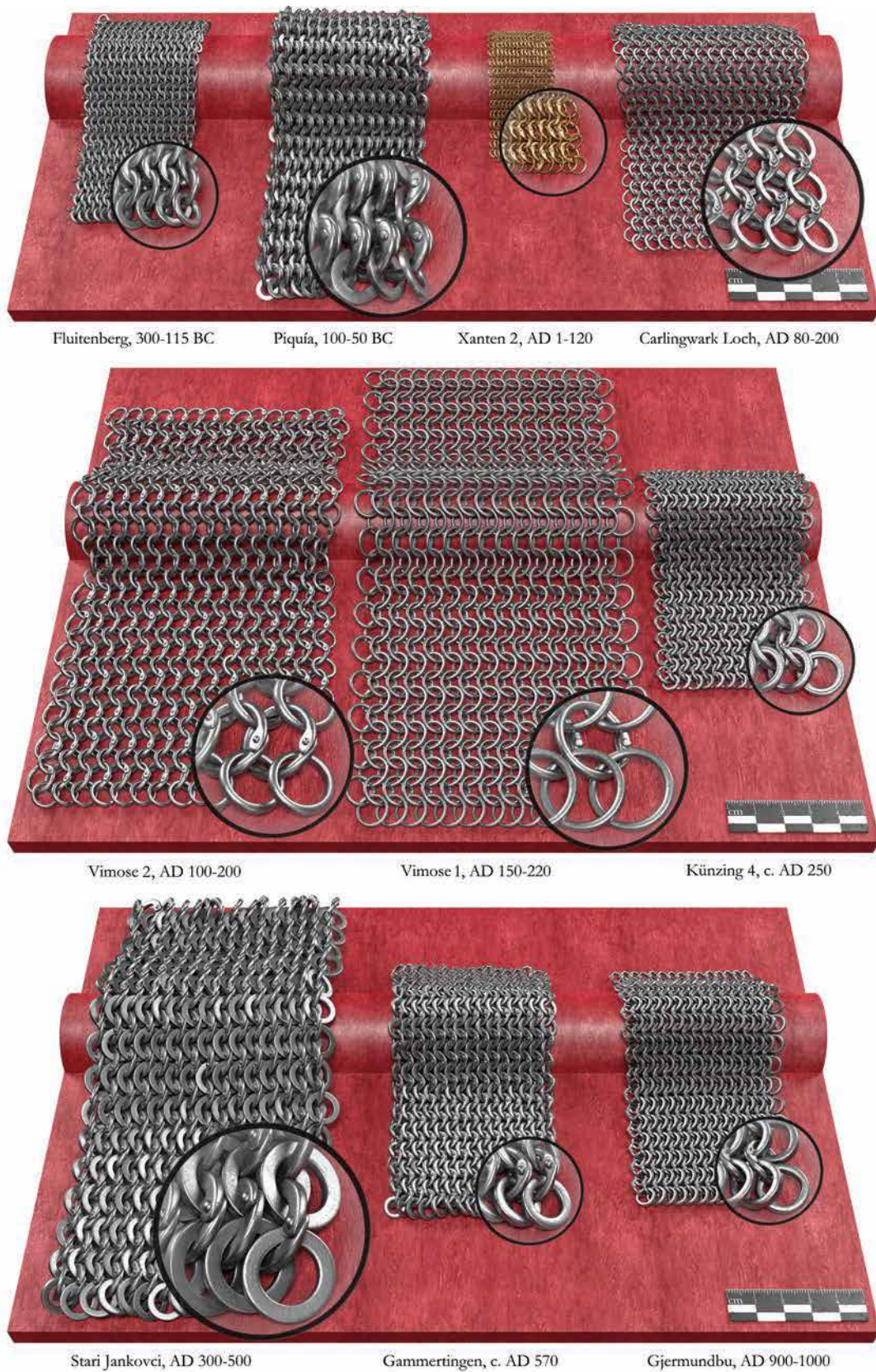
Fig. 11.1. Ten examples of mail meticulously recreated in virtual reality. Each fragment contains 30 rows of 15 rings, making a total of 450 rings per fragment. The ring characteristics, such as the outer diameter, directly affect the overall size of the fragment and the density of the fabric. The scale of the magnifying glass is 2.5x (drawing A. Moskvina and M. Moskvina).
