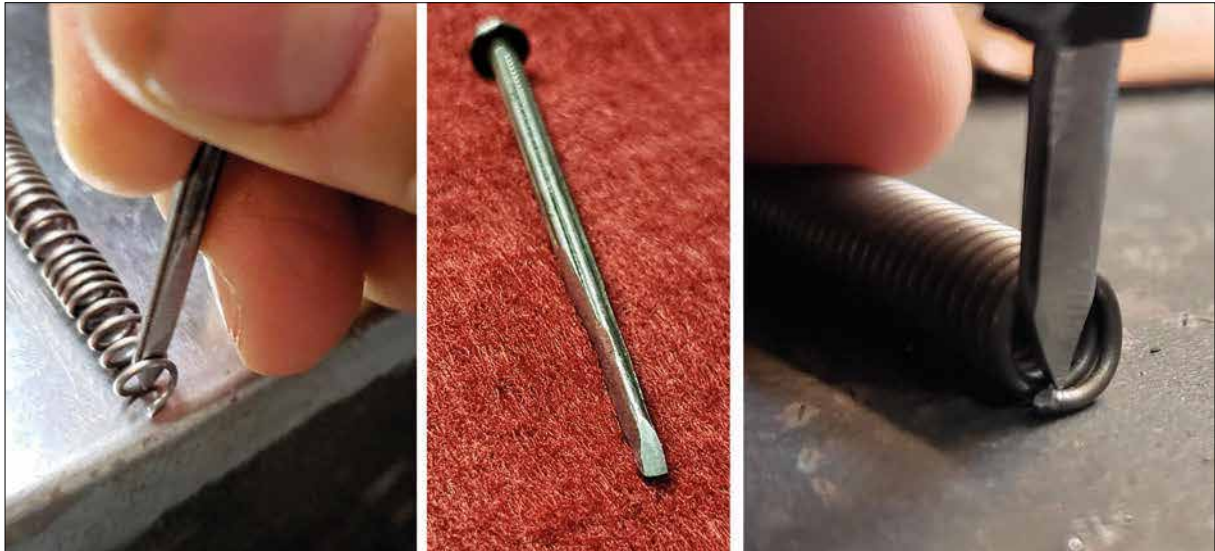
Fig. 11.28. Alfredo Mellace demonstrates here how rings can be cut from the coil with a small chisel. This method results in rings with an overlap shape found in the Roman mail of the Principate. The chisel, when sharp, will cut clean through the metal wire making an overlap with straight ends. As the chisel blunts, the end shape of the overlap changes to more rounded or pointed. During the Principate, mail has a very short stumpy overlap, probably due to how the rings were cut from the coil. On the left, the coil is opened in order to insert the chisel and make the overlap. In this manner, the length of the overlap can be as long or short as one desires. On the right, the links are cut without opening the coil. This is faster, as it omits a step, but has the disadvantage that it cuts down the length of the overlap to 2 mm, at most. The curvature of the rings does not allow a longer overlap with this method (photographs A. Mellace).
