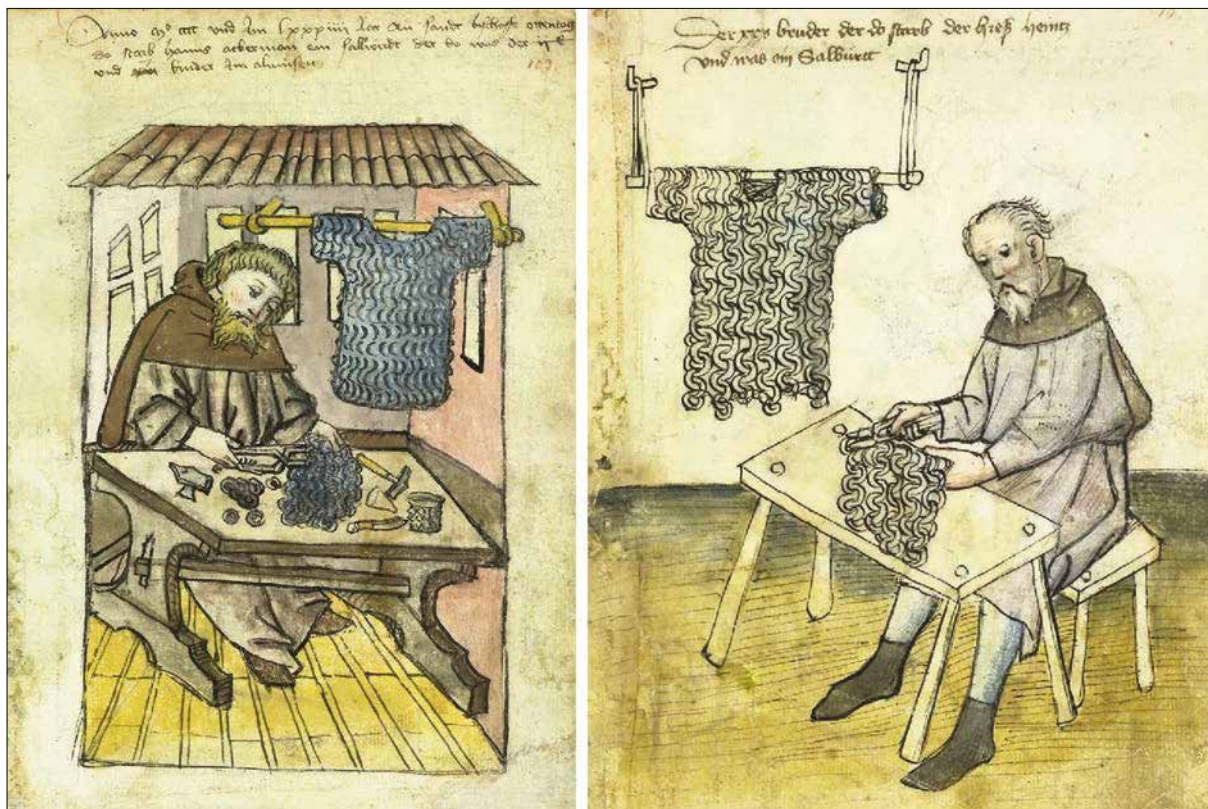
Fig. 8.3. Left: the mail maker Hanns Ackerman (died in AD 1484) surrounded by various tools of his trade. Besides the suspended beam which holds a mail shirt, we can see on his workbench a hammer, a small anvil, a knife, several loose rings and a glass. There is also the outline of an unidentified conical object. Hanns uses a pair of tongs to add rings to the segment he is working on. Right: the mail maker Heintz (died c. AD 1425) shown weaving mail while sitting on a bench. A wooden rod suspended by ropes is used to hang a mail shirt. Although the perspective is somewhat off, we can assume that, for practicality, the rod with the shirt was suspended above the workbench. Stadtbibliothek Nürnberg (MS Amb 317.2 – folio 9v & 103r).
